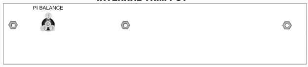
The TweedyDrive+ has 1 internal trim pot for the PI Balance – Useful for working with unmatched 12AX7 tubes in the phase inverter position. Refer to qualified personnel for proper setting.
