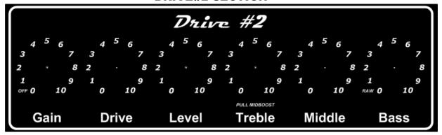
Because the amplifier sections are in series left to right, this section can be driven by the clean channel or the output of Drive #1. The section's range of effect is amazingly flexible because of its dedicated tone controls.
