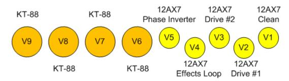
All tube brands are acceptable, a long plate is preferred in the V5 (Phase Inverter) position.
