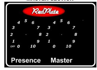
**Presence Control** – The presence circuit uses global negative feedback to remove low frequencies which frees up bandwidth for more midrange and highs. Think of it as a tone control to balance the relationship between highs and lows, especially when the amplifier is naturally producing increased low end at louder volumes. The control clicks off when rotated to zero for no presence.
