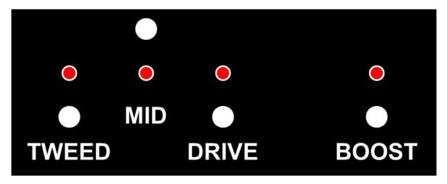
**TWEED** – When engaged (lit) the guitar input is routed to the Tweed channel. The footswitch button does not work when the Blackface Channel's volume control is pulled because it overrides the footswitch.
