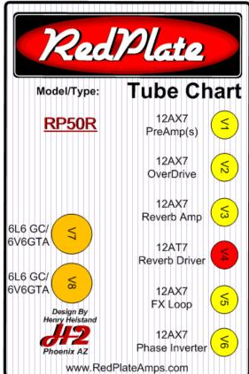
All tube brands are acceptable; a long plate is preferred in the Phase Inverter position. <u>CAUTION - NEVER MIX 6L6 AND 6V6 TUBES AND ALWAYS HAVE A SPEAKER</u> CONNECTED.
