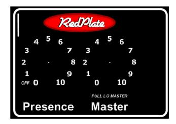
**Presence Control** – The presence circuit uses global negative feedback to remove low frequencies which frees up bandwidth for more midrange and highs. Think of it as a tone control to balance the relationship between highs and lows, especially when the amplifier is naturally producing increased low end at louder volumes. The control clicks off when rotated to zero for no presence.
