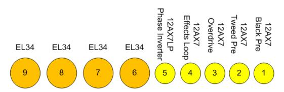
All tube brands are acceptable, a long plate is preferred in the V5 (Phase Inverter) position.
