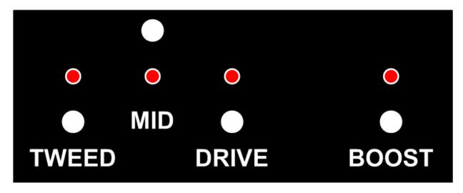
**TWEED** – When engaged the guitar input is routed to the Tweed channel. The footswitch button does not work when the Tweed Channel's Gain control is pulled because it is a duplicate function.
