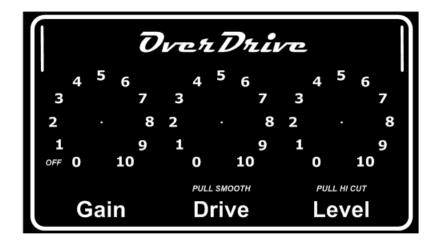
The OverDrive section controls the amount of character to add to the preamp tone. The section's range of effect can be just a hint of early break up or a full on aggressive Rock distortion.
