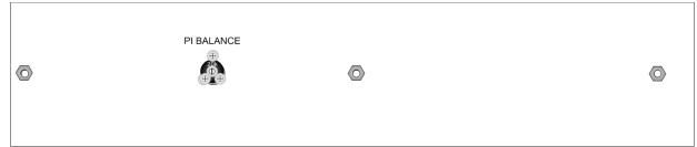
The OpenRange has an internal trim pot for the Phase Inverter tube balance – Useful for working with unmatched 12AX7 tubes in the phase inverter position. Refer to qualified personnel for proper setting.
