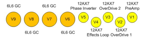
All tube brands are acceptable, a long plate is preferred in the V5 (Phase Inverter) position.
