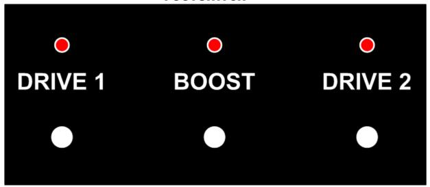
**DRIVE 1** - The indicator comes on when the Drive #1 section is active. The footswitch button does not work when the front panel Drive #1 Gain control is rotated to zero because it is a duplicate function.
