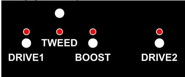
**TWEED** – Same as rotating the MODE control to TWEED for immediate access to the fattest preamp tone. This button has no effect when the MODE control is already in TWEED position
