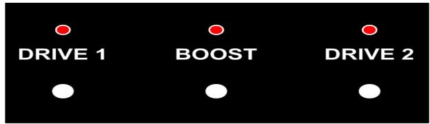
**DRIVE 1** - The indicator comes on when the Drive #1 section is active. The footswitch button does not work when the front panel Drive #1 Gain control is rotated to zero because it is a duplicate function.
