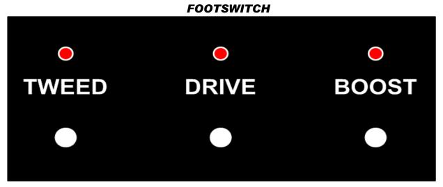
**TWEED** - Same as rotating the Mode switch to position 6, for a traditional fat tweed tone. The footswitch button has no effect when position 6 of the rotary MODE switch on the front panel is selected because it is a duplicate function.
