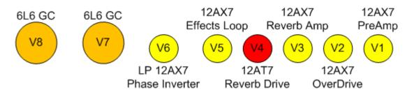
All tube brands are acceptable, a long plate is preferred in the V6 (Phase Inverter) position.
