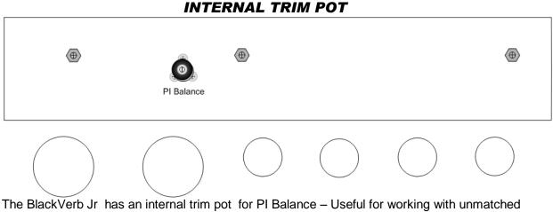
The BlackVerb Jr has an internal trim pot for PI Balance – Useful for working with unmatched 12AX7 tubes in the phase inverter position. Refer to qualified personnel for proper setting.
