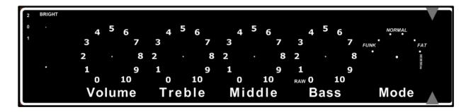
The Clean Preamp is designed to imitate (and surpass) all of the "classic" guitar amp preamps. The BlackLoop Mode control gives the player the ability to shift midrange center point frequency.
